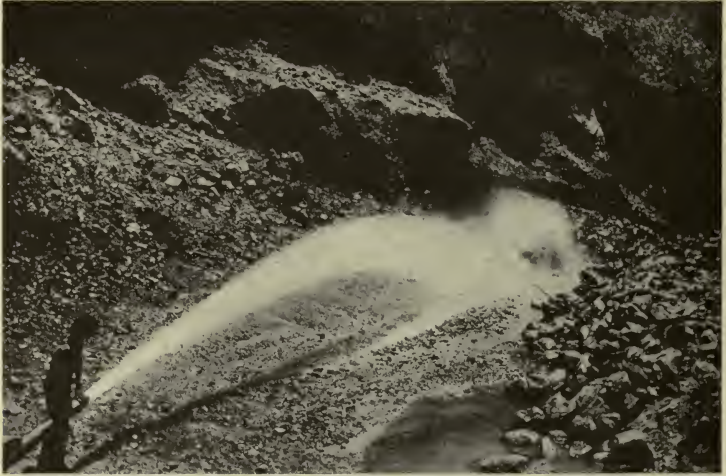
FIG. 100.—HYDRAULIC MINING ON THE KLAMATH RIVER, CALIFORNIA
